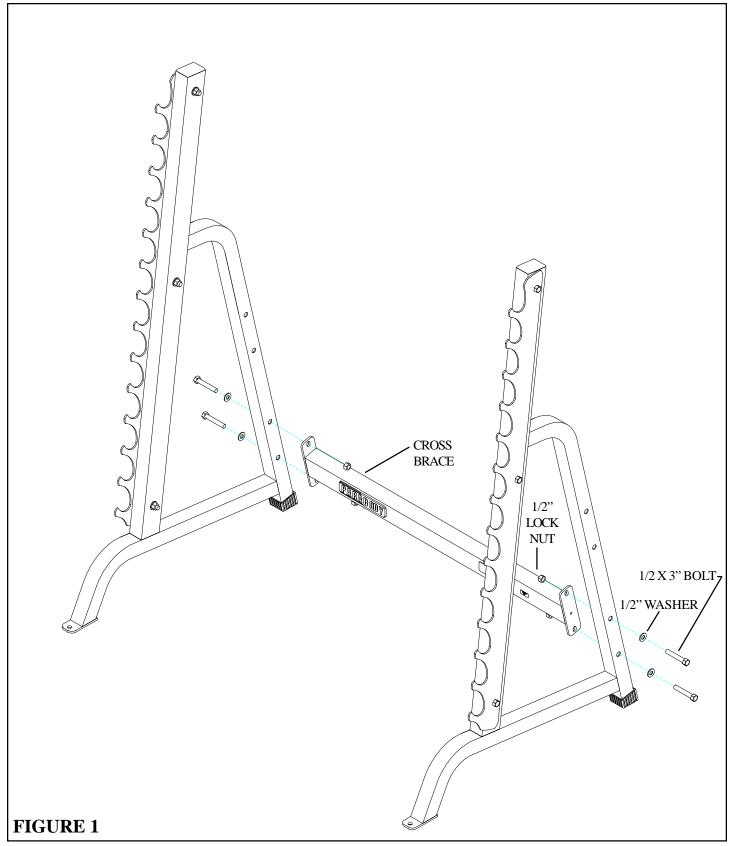
STEP 1: INSTALLATION SHOWN FOR 838 SQUAT MACHINE. 888 SMITH MACHINE INSTALLATION SHOWN ON PAGE 4 & 5.
